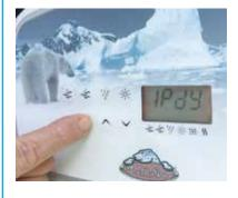
Step 3. Scroll to next LLP Setting to view the Spas IP Address Assigned as Displayed on the Topside Controller.
